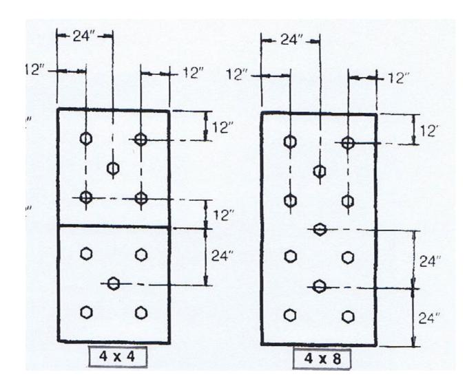
Figure 1. Insulation Fastening Patterns
