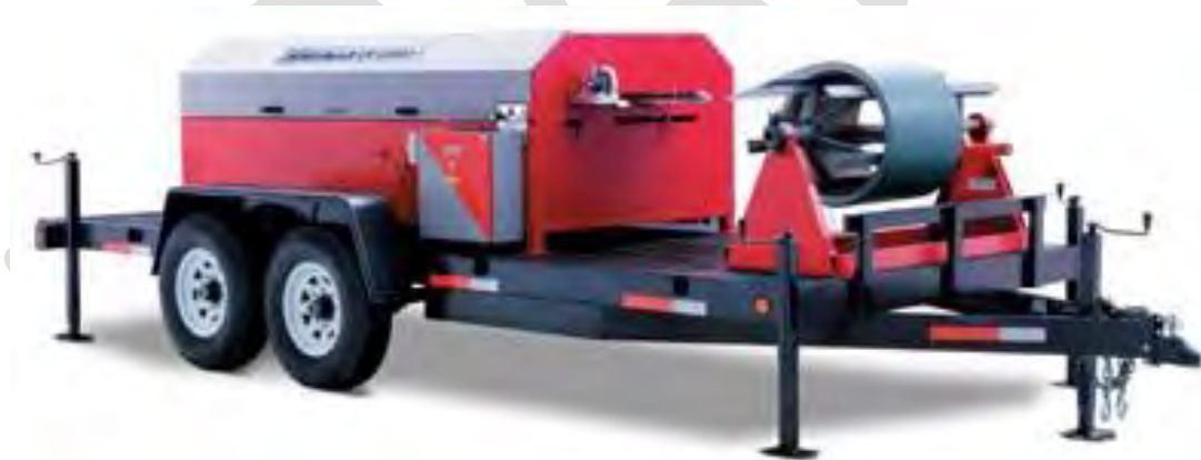
Figure 2: Mobile Roll Former (Photo courtesy Schlebach Machines)
