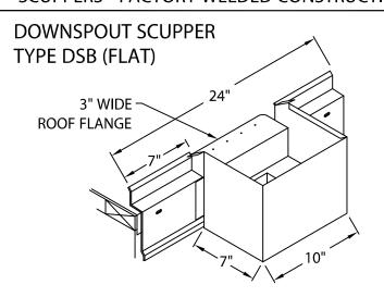
FOR USE WITHOUT TAPERED EDGE STRIP. FLANGE FLUSH MOUNTED WITH ROOF.
