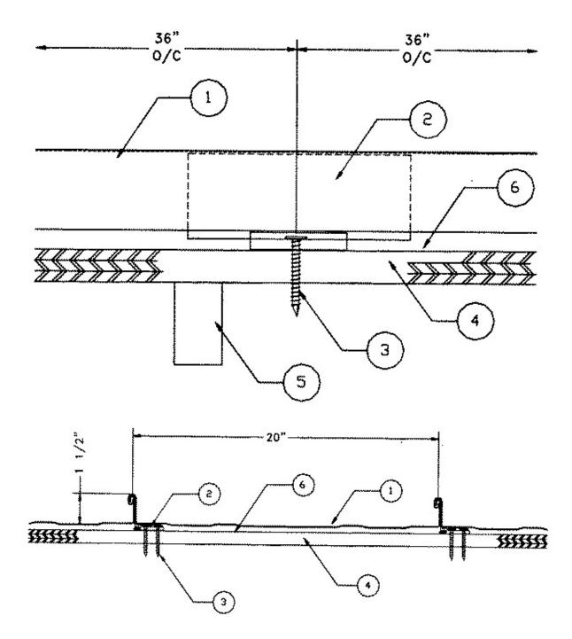
1. Metal Roof Deck Panels\* — Min. 0.032 in. thick embossed aluminum; width 20 in. max., height of female rib 1-1/2 in., male rib 1-29/64 in. Panels continuous over three or more clips with no end-laps. A bead of sealant may be used at panel ribs. Panel ribs seamed with an electric seamer with seaming operation to include upper portion of panel clip (Item 2).
