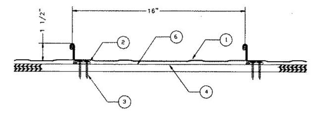
1. **Metal Roof Deck Panels\*** — Min. 24 MSG (.0225 in.) thick coated steel; width 16 in. max., height of female rib 1-1/2 in., male rib 1-29/64 in. Panels continuous over three or more clips with no end-laps. A bead of sealant may be used at panel ribs. Panel ribs seamed with an electric seamer with seaming operation to include upper portion of panel Clip (Item 2).
