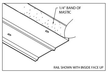
2. Miter & Scupper Base Rail (Preparation) Lay miters and spillout scuppers on deck with outside face down. Be sure aluminum base rail is clean and free of dirt or dust. Apply a heavy 1/4" (6 mm) band of approved mastic/sealant to the back of the deck flange to entire length of rail as shown. Application of sealant is required along the full length of each miter base rail.
