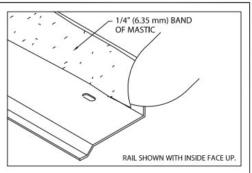
2. Miter & Scupper Base Rail (Preparation) Lay miters and spillout scuppers on deck with outside face down. Be sure aluminum base rail is clean and free of dirt or dust. Apply a heavy 1/4" (6 mm) band of approved mastic/sealant to the back of the deck flange to entire length of base rail as shown. Application of sealant is required along the full length of each miter base rail.
