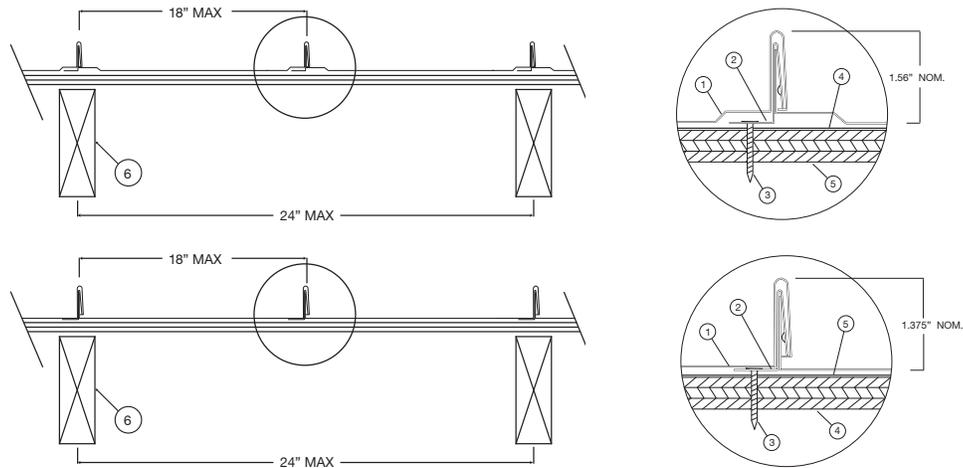
**1 Metal Roof Deck Panels \* / “Redi-Roof Standing Seam”**
