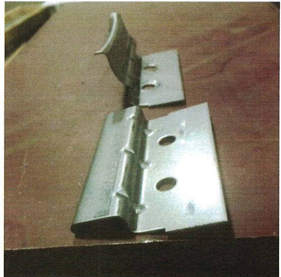
TYPICAL CLIP WITH TYPICAL FAILED CLIP
