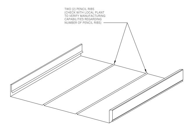
SNAP-CLAD PANEL WITH PENCIL RIBS ISOMETRIC VIEW
