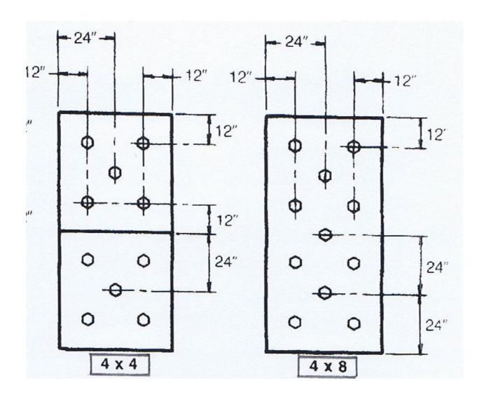
Figure 1. Insulation Fastening Patterns
