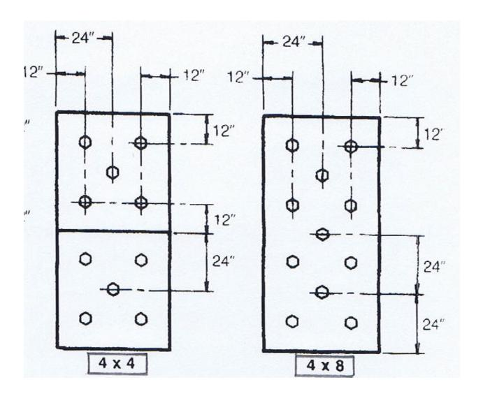
Figure 1. Insulation Fastening Patterns
