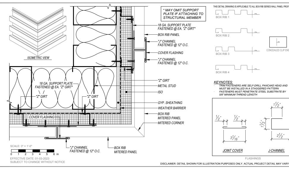
BOX RIB 1 BOX RIB 2 -CONCEALED CLIP END BOX RIB 3
