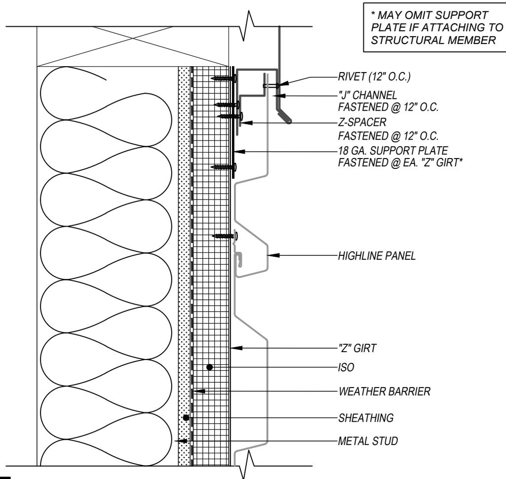
THIS DETAIL DRAWING IS APPLICABLE TO ALL HIGHLINE SERIES WALL PANEL PROFILES
