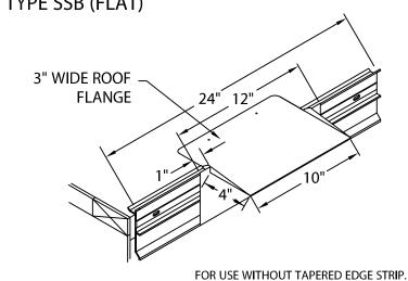
FOR USE WITHOUT TAPERED EDGE STRIP. FLANGE FLUSH MOUNTED WITH ROOF.
